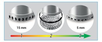
The **DR steel** easily converts from an ordinary submersible pump to a *dry floor* unit. When operating in this mode, the suction level can be reduced to as little as **5 mm** above the ground.
