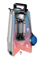
The cooling jacket ensures an optimal **motor** temperature even with the pump only partially submerged.
